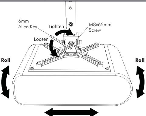
To make Roll/Shift adjustments, first ensure the weight of the projector is supported. Then loosen the M8x65mm Screw with the supplied 6mm Allen Key, and adjust to your desired position. Re-tighten the screw firmly.
