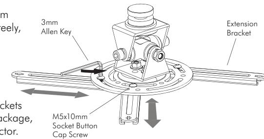
You may need to replace the attached Extension Brackets with the additional longer brackets supplied in the package, to suit the mounting hole configuration of your projector.
