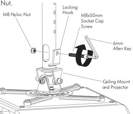
**Tip:** When the projector requires servicing, remove the projector via this easy disconnection point to save time.
