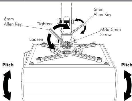
To make Pitch adjustment, first ensure the weight of the projector is supported. Then loosen both M8x15mm Screws with the supplied 6mm Allen Key, and adjust to your desired position. Re-tighten both screws firmly.
